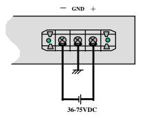
Figure B4.1: 48 VDC Terminal Block on Magnum 508/528/528F-48VDC models
